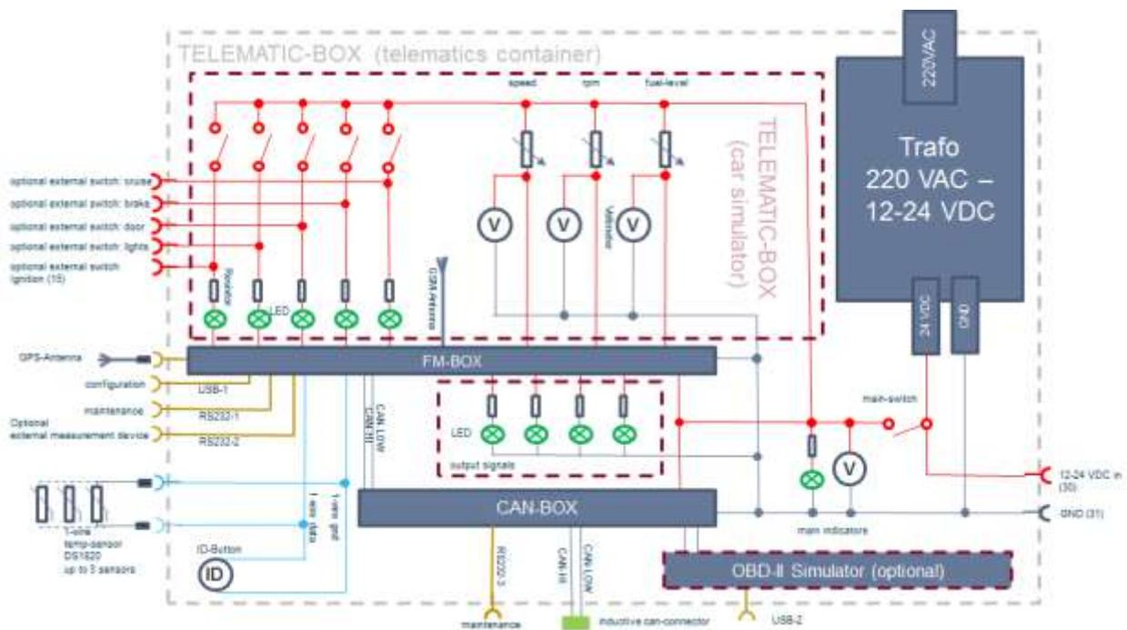
Fig. 0.5: Schematic Wiring, Switchboard and External Connectors
