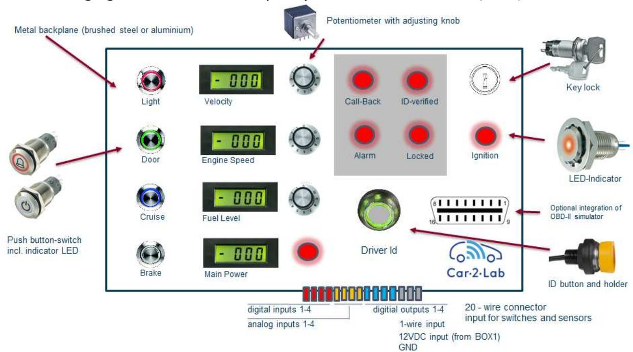
Fig. 0.7: Sample Layout of the Car Simulator
